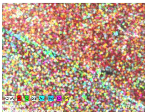
Figure 6. EDX analysis of the treated surface of the probe
